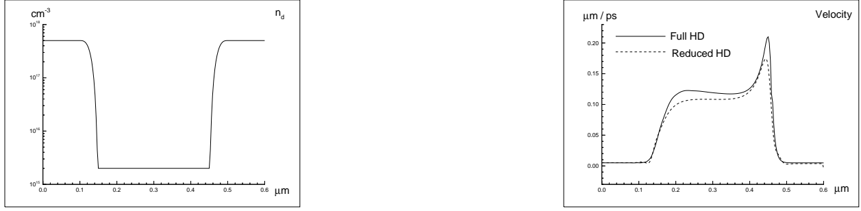
FIG. 5.13. The one dimensional n^+ - n - n^+ channel. Left: the doping n_d ; Right: the velocity v , comparison of the HD model and the reduced HD model.
