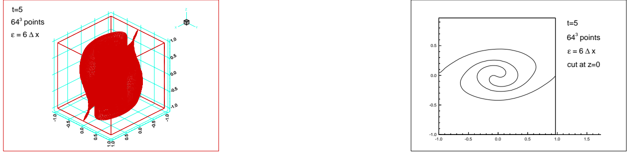
FIG. 5.12. Three dimensional vortex sheet simulation. t = 5 . ENO with 64^3 points. \delta function width \epsilon = 6\Delta x . Left: three dimensional level surface; Right: z = 0 plane cut.
