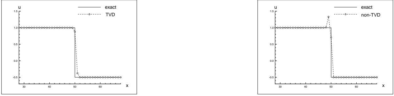
FIG. 4.1. Second order TVD MUSCL spatial discretization. Solution after 500 time steps. Left: TVD time discretization (4.10); Right: non-TVD time discretization (4.22).
